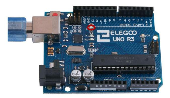
You may find that your UNO R3 board's 'L' LED already blinks when you connect it to a USB plug. This is because the boards are generally shipped with the 'Blink' sketch pre-installed.
