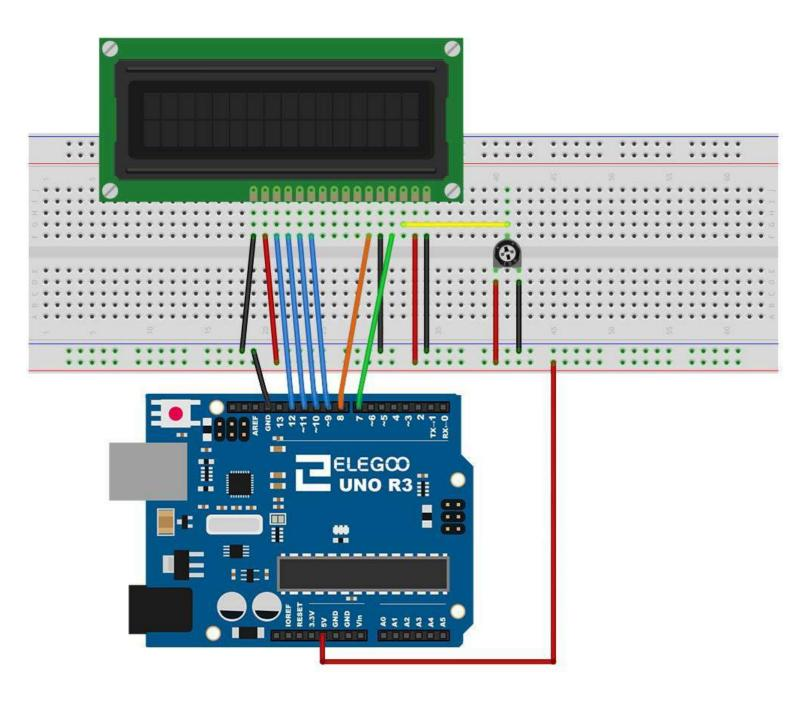
The LCD display needs six Arduino pins, all set to be digital outputs. It also needs 5V and GND connections.
